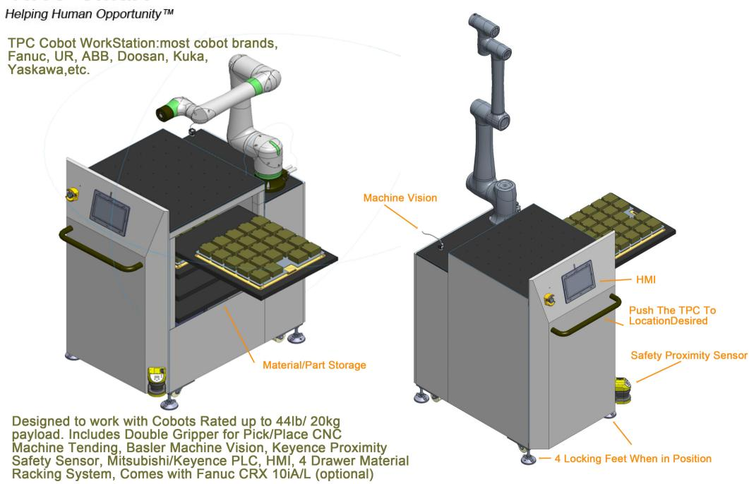
TPC is an economic, efficient CNC Machine Tending Mobile Work Station for use with a Cobot. Use at 1 primary machine location or move between several machines to maximize the cobot workload for quicker ROI as needed! The 4 drawer racking system can store both material blanks and finished workpieces. Ideal for small-medium sized parts.
