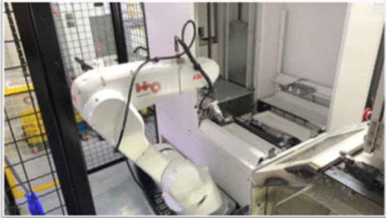
Robot Arm With Adjustable Positioning for Pick/Place and to Create Additional Space When not in Use.
